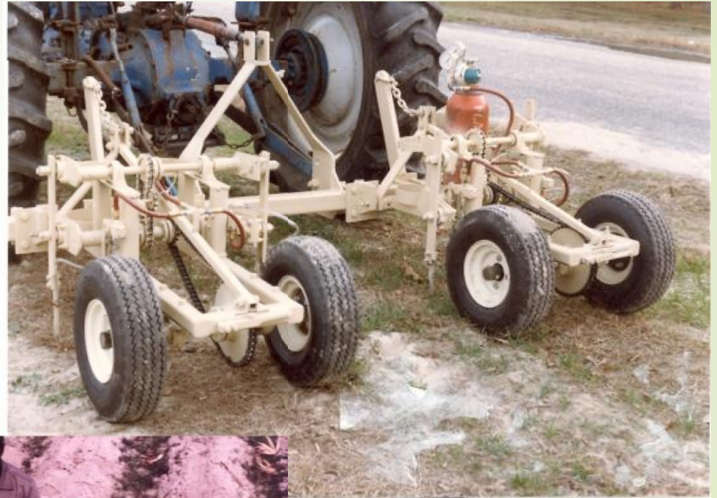
Sewing Machine Type Injector for Lawns and Gardens
